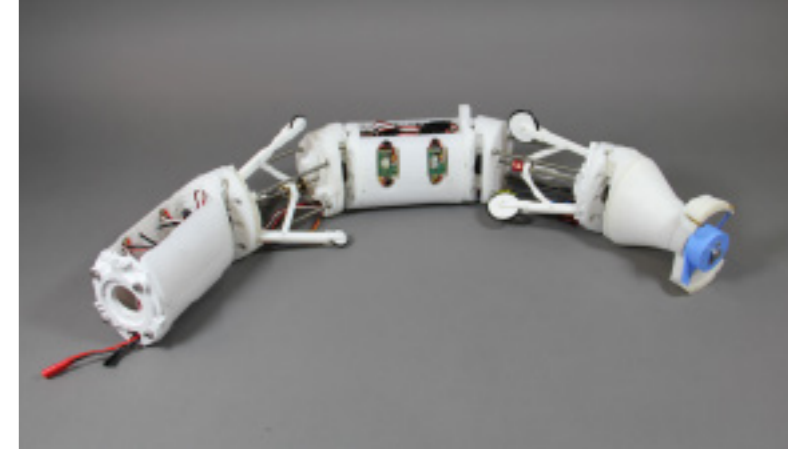
Prototype of an autonomous inspection robot (AIR) that remains in the pipeline for a long period of time and charts the state and location of smaller pipes
